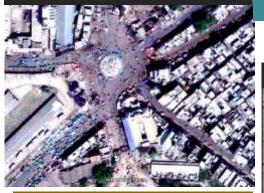
Major Issues •Very high pedestrian movement •Important bus/IPT terminal with no designated bus stops and halt bays •Rear entry to the Railway Station right at the intersection •Absence of proper road marking •Absence of necessary channelizers
