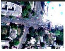
Major Issues •Absence of proper road marking •Absence of necessary channelizers •Footover bridge only present on one arm •Signals not in use •Haphazard halting/parking of IPT modes and private vehicles •Poor enforcement techniques
