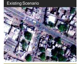
**Major Issues** •Significant movement of freight movement on slow moving vehicles and animal carts •Absence of proper road marking Absence of necessary channelizers •Lack of pedestrian facilities •Signals not in use Haphazard halting/parking of IPT modes and Buses Poor enforcement techniques
